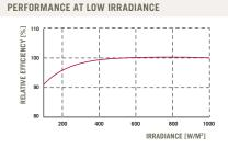
Typical module performance under low irradiance conditions in comparison to STC conditions ( $25\,^{\circ}$ C, 1000 W/m<sup>2</sup>).
